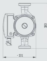
7.0 m 3.900 l/h 4 - 42 W 4 constant characteristics, 4 proportional characteristics, Air vent program, Keylock 1x 230V, 50 Hz No external motor protection required IP 42 0 °C to +40 °C +5 ℃ to +110 ℃ TF 110 as per CEN 335-2-51 10 bar DN 15, DN 20, DN 25, DN 32 110 mm, 130 mm, 180 mm 130 mm, 180 mm variant in grey cast iron cataphoresis coated; 110 mm variant in brass 2.5 kg ≤0.15
